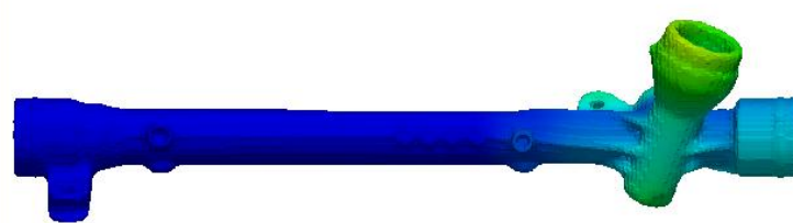
Couple: shrinkage + gas porosity
