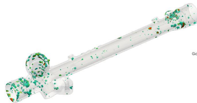
Gas blocked in the casting
