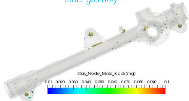
Shrinkage porosity and gas porosity
